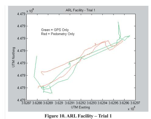
The first run conducted in the ARL Robotics Facility used a "Regular Walking" pace. Most of the trial, with the exception of the beginning and end, was conducted inside of a building, making the GPS data of extremely poor quality. The pedometry data more closely resembled the true path traveled than did the GPS data.
