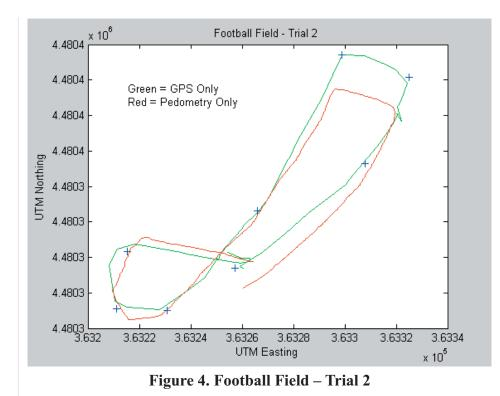
Trial 2 of the Football Field course used a fast walking pace. A rough and notably sparse GPS signal persisted throughout the entire run. In addition, the tester tripped at one point during the middle of the run causing a brief amount of poor pedometry data.
