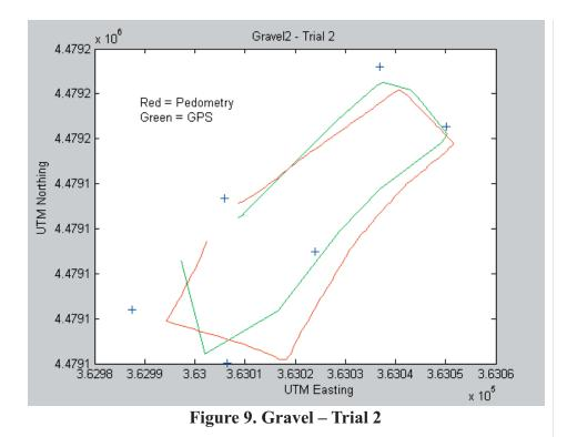
Trial 2 of the Gravel course used a "Regular Walking" pace. The run was relatively uneventful with the exception that poor quality GPS data was observed toward the end of the run. In fact, in this case the path traced by the pedometry output more closely resembles the path walked by the tester.
