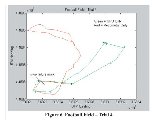
A jogging pace was used during Trial 4 of the Football Field course. Gyro failure occurred fairly early on in this trial, making much of the later data unreliable. The tester also stopped for a short rest from jogging near flag point 6. However, this anomaly is overshadowed by the erroneous data caused by the failed gyro.
