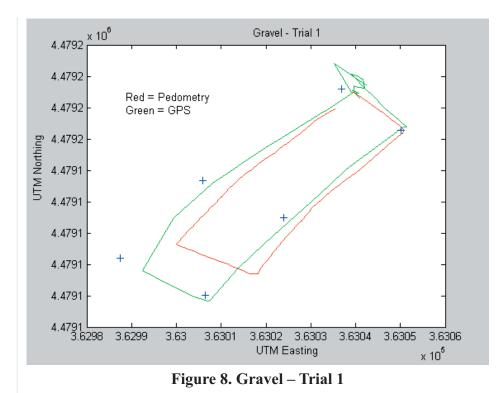
Trial 1 of the Gravel course used a slow to moderate walking pace. Poor quality GPS data was observed during the beginning of the run, but most of the trial went according to plan.
