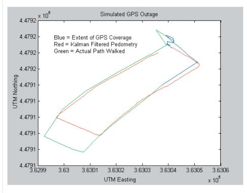
Figure 15. System with Simulated Outages on Gravel Pit
