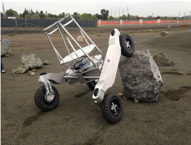
Figure 13: KReX2 exercising the differencing bar to maintain terrain contact for all wheels.
