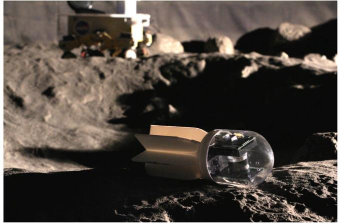
Fig. 2. Miniaturized prototype microscope installed as a rover-deployed projectile payload, demonstrating a remote sensor concept for hazardous terrain inaccessible to the parent vehicle.
